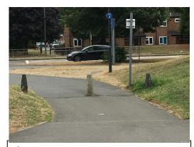
Small bollards with low contrast and no reflective bands are hard to see, making them a dangerous obstacle for path users
